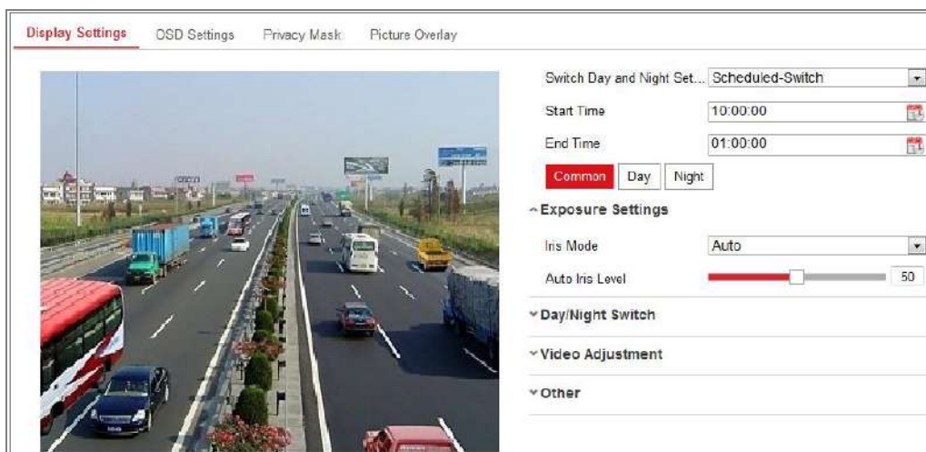
Figure 9-5 Day/Night Scheduled-Switch Configuration Interface
